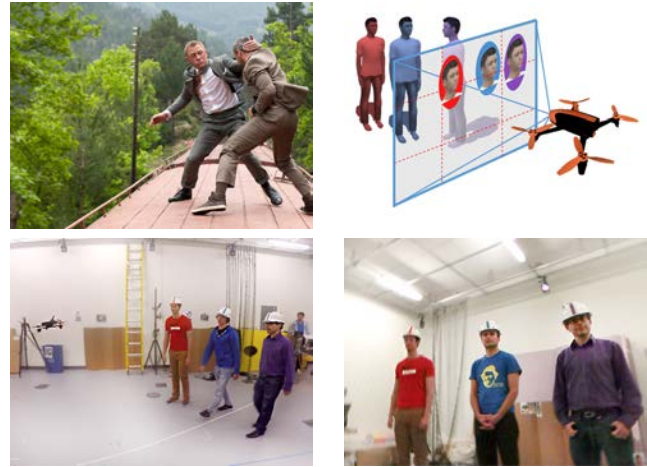
Fig. 1: We propose a real-time method to film shots of dynamic scenes automatically. The user specifies target positions on screen. We solve for robot trajectories and gimbal controls, producing footage that adheres to aesthetic constraints, minimizes visual occlusion and produces collision-free trajectories in dynamic scenes.
