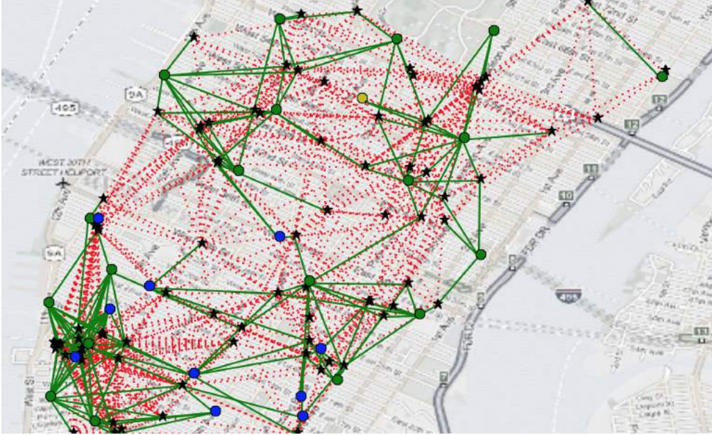
Fig. 3. Example of a pairwise RV-graph for 90 requests (star) and 30 vehicles (circle) with edges between two requests in dotted red and between a request and a vehicle in solid green. The maximum waiting time and delay are three and six minutes in this example.
